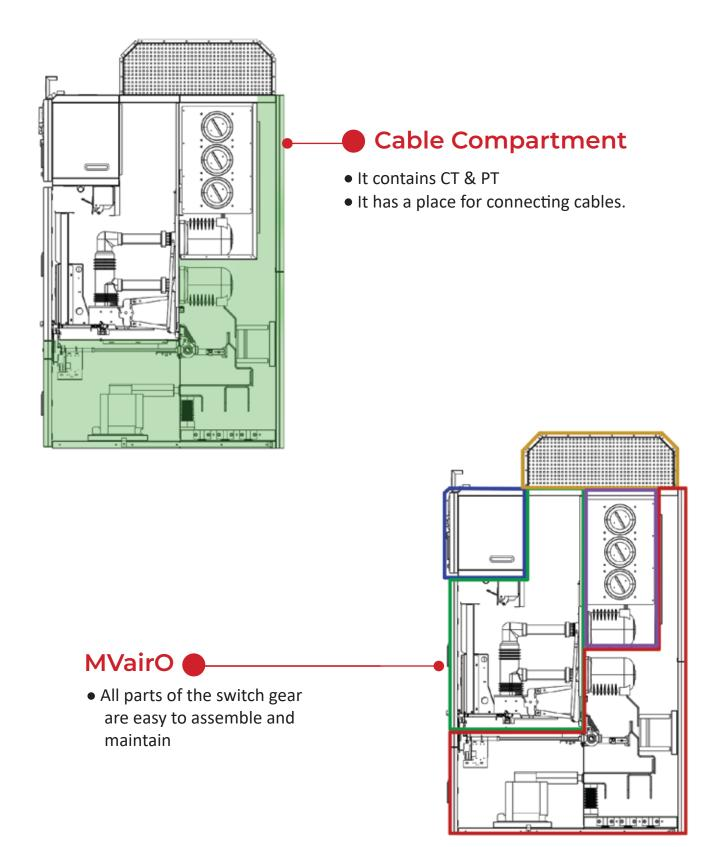
MVairO is medium voltage switchgear with a metal enclosure, suitable for indoor installations. Metal partitions segregate the compartments from each other and the live parts are air-insulated. The main technical characteristics are shown as follows:
